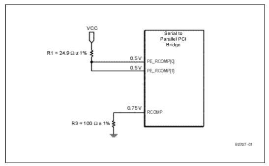
Figure 25. Reference and Compensation Circuit Implementations
